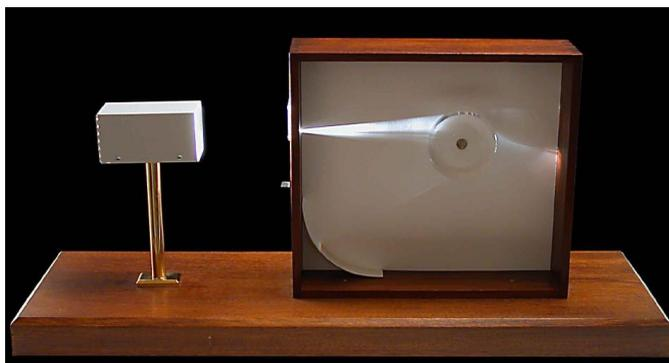
Experimental Setup by Kamāl al-Dīn al-Fārisī (ca. 1300 ce) to demonstrate the generation of the rainbow by double refraction and one or two reflections of the sunlight in the raindrop. The model was made after his description.
